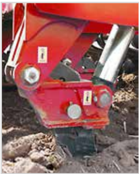
The Pro-Lift tine as hydraulic auto-reset version available on DTX.
